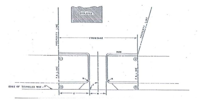
Illustration 3: Driveways for Corner Installations Diagrammatic For Illustrating Definitions
